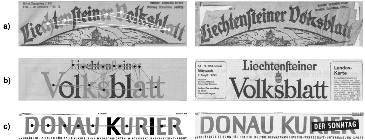
Figure 1. Three front page graph models, each with a correctly recognized candidate, illustrating: a) limited distortion resilience; b) scaling invariance; c) occlusion.
