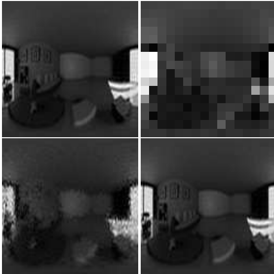
Figure 2: Groundtruth high-resolution image (top-left), one low-resolution image (top-right), reconstructed image with registration errors (bottom-left), reconstructed image with the proposed algorithm (bottom-right).
