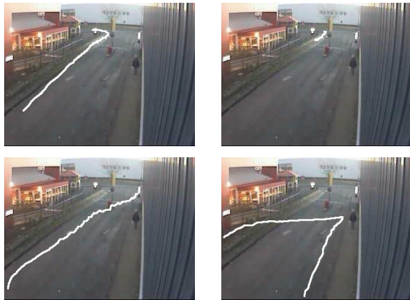
Figure 3: Results of p\text{-dtw} on the video. The first two pictures show common trajectories, while the last ones are detected as being rare, with only one occurrence for each model.
