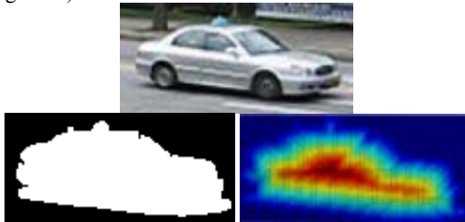
Figure 1. The original image (top), the detected image mask (bottom left) and the constructed kernel (bottom right).
