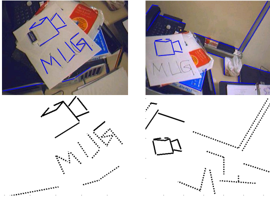
Figure 3: Comparing object and background cluster densities. Top: Images with overlaid test lines. Bottom-left: Density of clusters d(Object) = 1.76, d(Bkgrnd) = 1.56 . The small difference in values is due to the structural similarities between mug shape and the background (e.g. alphabet U, G etc.). Bottom-right d(Object) = 2.37, d(Bkgrnd) = 0.06 ; the object forms a much stronger cluster than the background.
