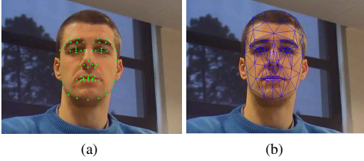
Figure 3: (a) Features Detection (b) Mesh Initialization
